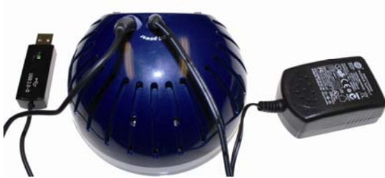
Fig. 5: Rear side of the Wöhler CDL 210 with USB cable and power supply
